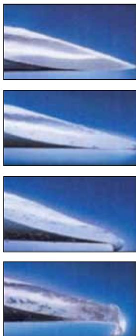
Figure 1. Reuse of insulin needle resulting in a hook shape.
